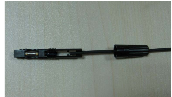
9、 Screw off the tail sleeve, and take off the cable.
