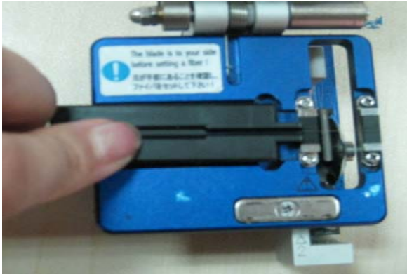
4、 Cut the cable to 10mm
