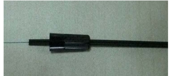
3、 Put the tail sleeve into the cable sheath
